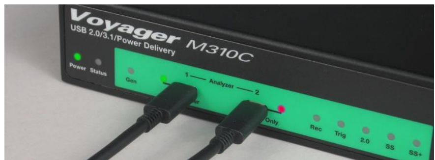
Diagram 1: The right cable here is plugged in incorrectly. It should be flipped, so that the LED turns green.
